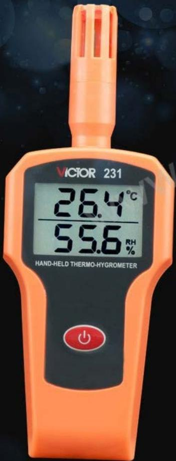
The image shows a handheld thermo-hygrometer, model VICTOR 231. It is orange and black. The digital display shows a temperature of 26.4°C and a relative humidity of 55.6 RH%. The device has a power button at the bottom and a sensor probe at the top. The background is dark with a bokeh effect.
